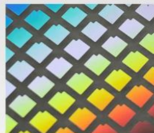
Actual photo of 1200V vertical GaN FETs currently in fab
