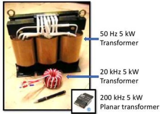
Examples of Passive Components Accompanying Switches
